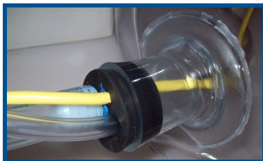
Extra Port for Anaerobic Gas Infuser located behind the airlock on all new Coy Anaerobic Chambers
